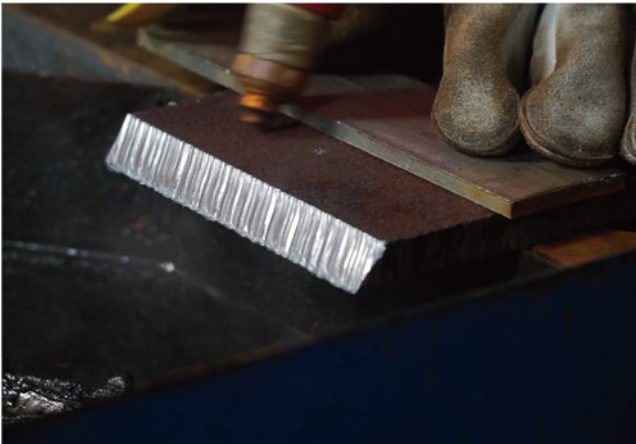
*16mm M.S. 60° bevel cutting by PROCUT-75MAX
